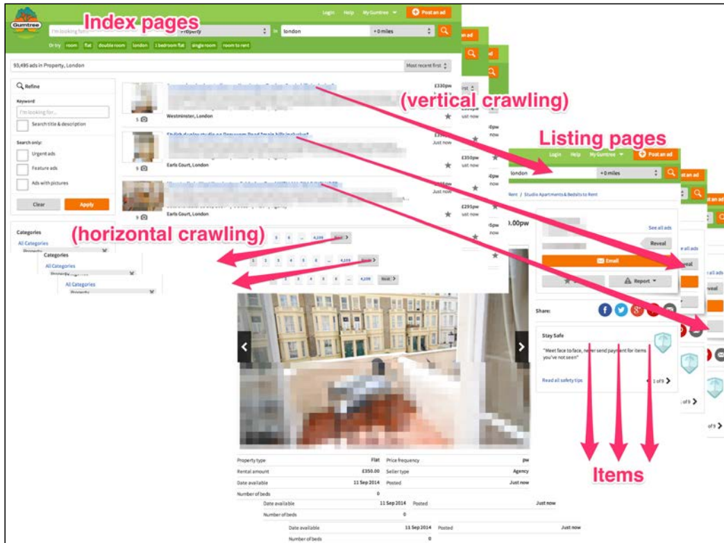
A typical crawler moves in two directions
